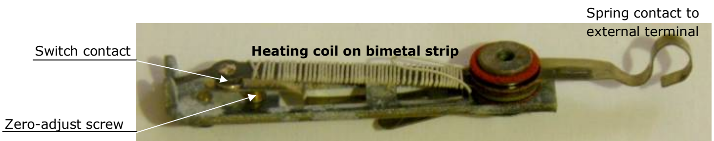
Figure 7: Bimetal temperature sensing element (Aftermarket unit but similar to Smiths sender.)
