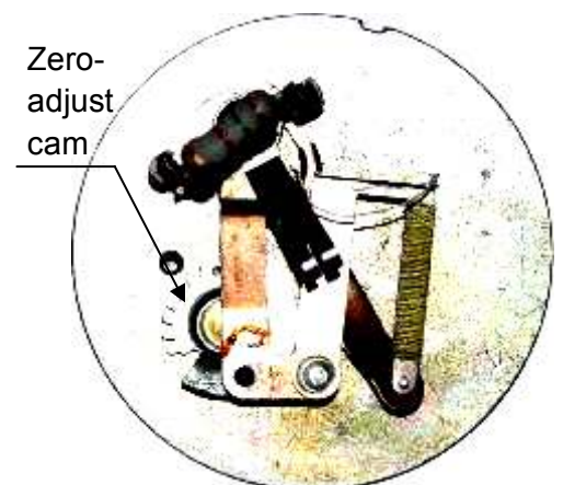
Figure 21: Bimetal pressure sender internals.
