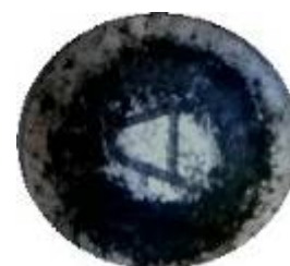
Figure 13: Damaged thermistor disc,
