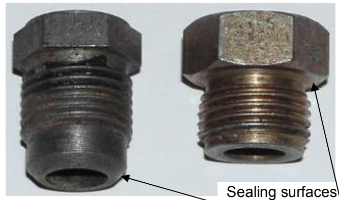
Figure 15: The difference between a TT380x and TT480x is in the collar – TT380x on left, TT480x on right.
