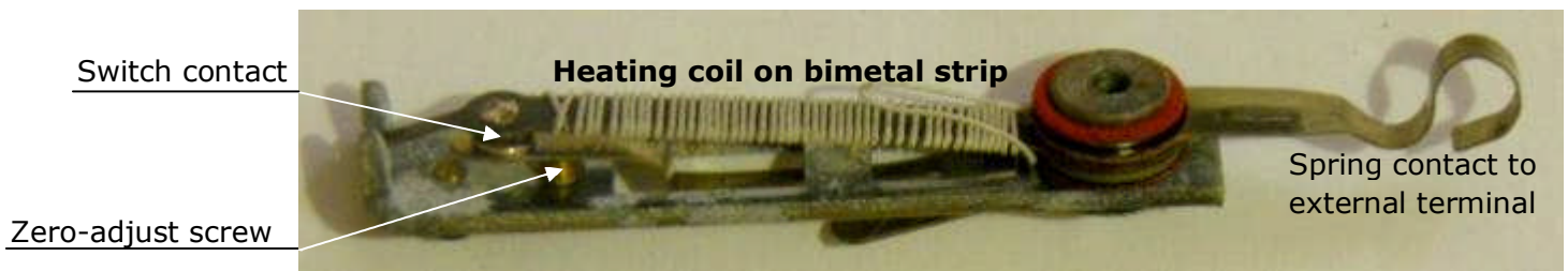
Figure 7: Bimetal temperature sensing element (Aftermarket unit but similar to Smiths sender.)
