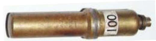
Figure 5: Smiths TT 1200/01 bimetal temperature sender.
