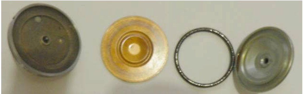
Figure. 22: Lower portion of bimetal pressure transmitter .
