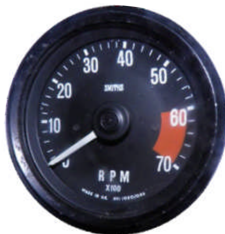
FIGURE 4.1: Typical Gen-2 OEM tachometer.
