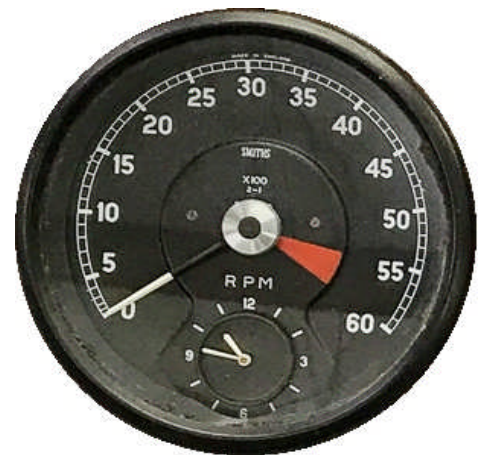
FIGURE F.3: Typical Smiths RV 7000 series tachometer. This one a RV 7403/00 from a 1962 Mk. II Jaguar. Photograph by Phil Turnbull, NZ
