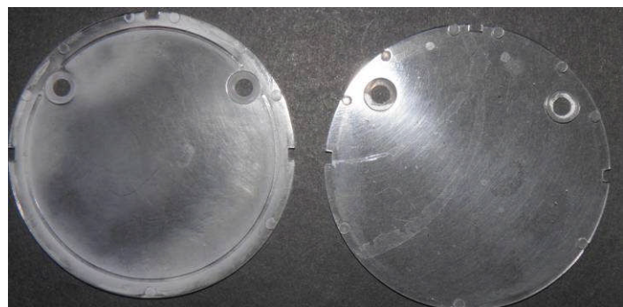
FIGURE 6.13: showing partially polished clock glasses. Glass with raised ring on left. Plain glass on right.
