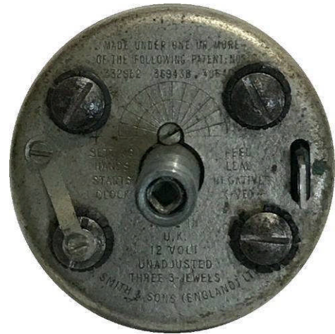
FIGURE 5.1: Rear view of a Smiths CE “rear adjust” car clock. The rectangular pattern of the mounting screws identifies the CE type movement.
