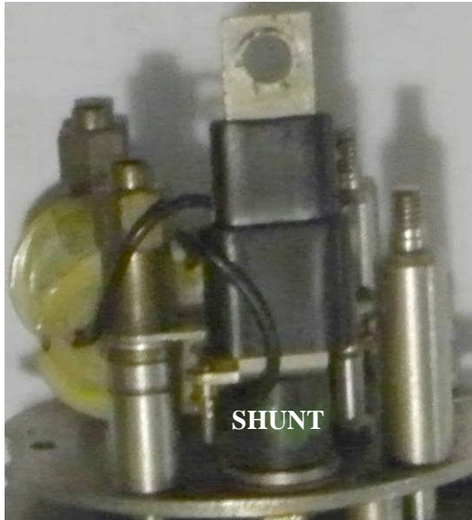
FIGURE 5.5a: Partly dismantled Smiths 12V CE clock movement (Yellow insulation tape on coil) with black shunt resistor fitted. Note also the Black insulating sleeve on the input terminal bracket.
