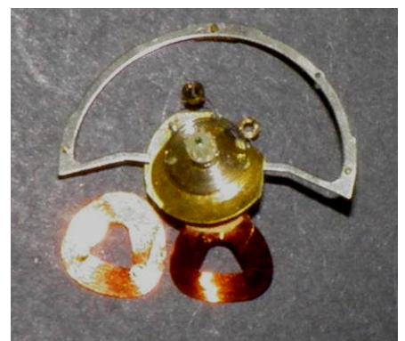
FIGURE 6.2: Damaged balance wheel assembly as removed from Smiths CTE clock.
