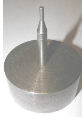
FIGURE 1.13: Cross sectional sketch of minute hand and boss showing the final position of the centre spindle (grey) within it. Photograph on right is a purpose-made anvil to support the centre spindle when fitting the minute hand assembly. (Refer Fig. 1.12 above.)
