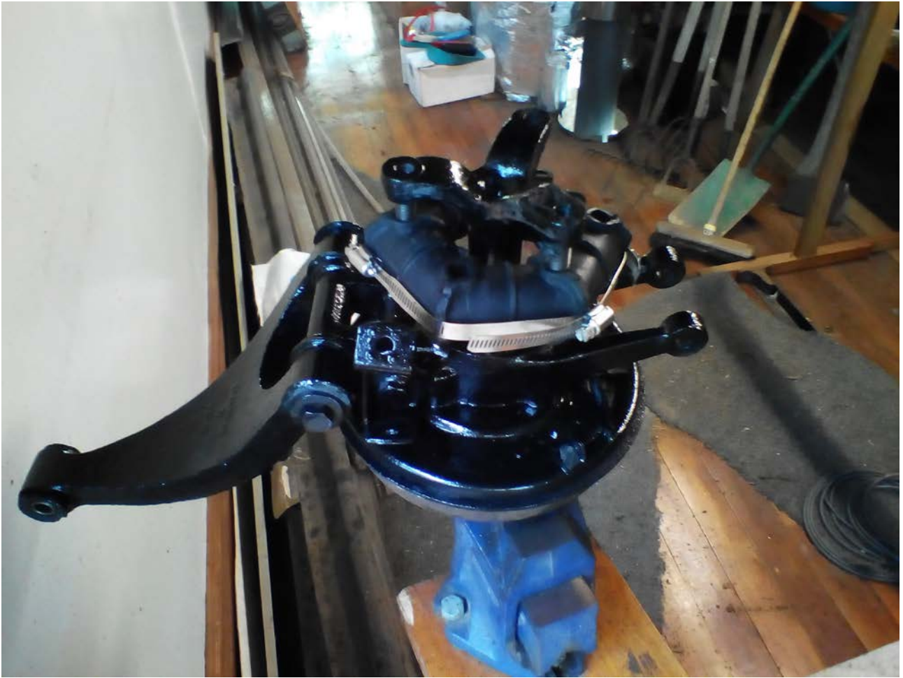
Figure 7: one bolt started (left) and a second's untreaded tip inserted into outer driveshaft
