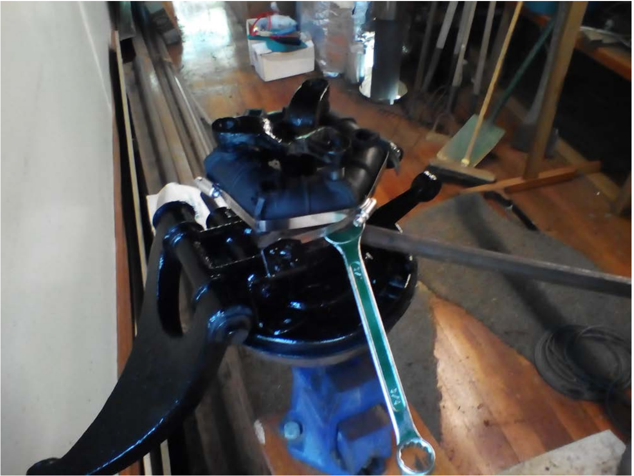
Figure 8: upward pressure to start bolt in threads
