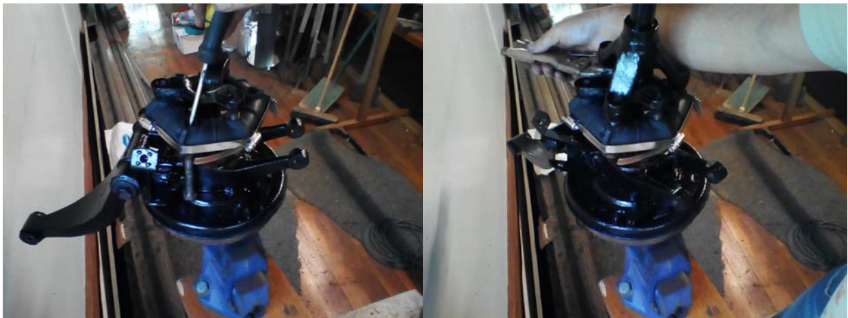
Figure 9: straightening donut to accept a bolt Figure 10: levering a bolt with vise grips
