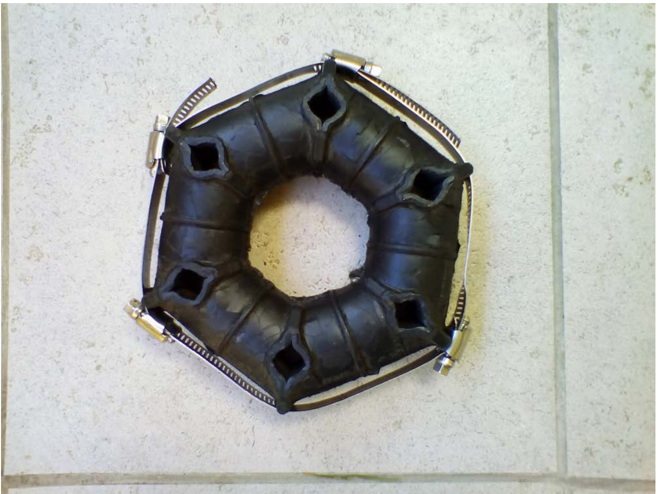
Figure 6: donut with jubilee band tensioners at corners
