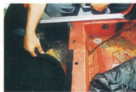
Rear suspension mounts can pull through floorpan if unchecked. Lift out seat to see.
