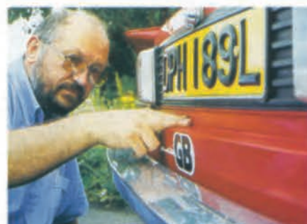
Seam just below rear light panel harbours rust, eventually causing boot to leak too.
