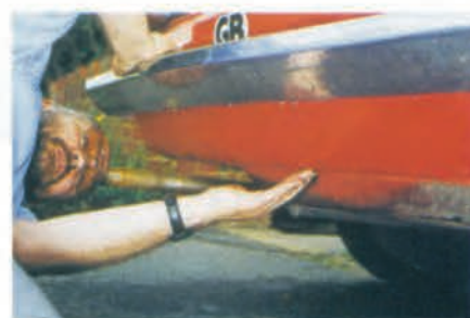
Rear valance acts as a mud trap, causing it to rot from behind. Needs regular clean.
