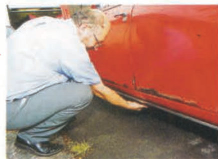
Sills rot readily but are crucial to the car's strength and rigidity. Check them carefully.
