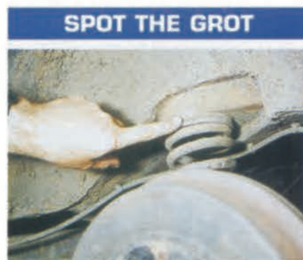
Rear spring mounting can pull away from the inner wheelarch, so check it carefully.
