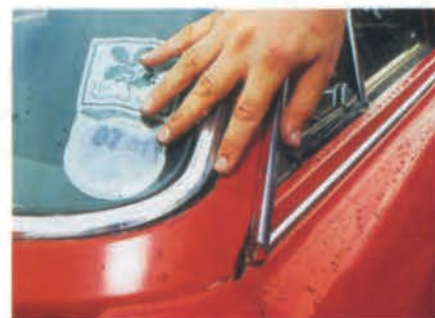
A-post dissolves around the windscreen aperture and at the base of the rain gutter.
