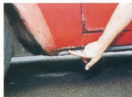
Trailing edge of front wing and surrounding area rot if drain holes become blocked.
