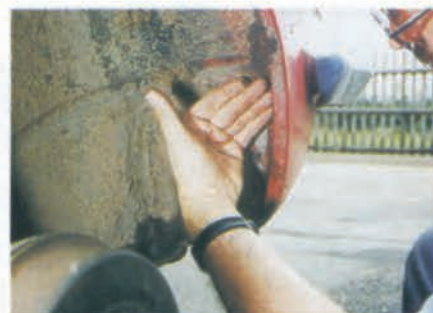
Rear inner arch often rots badly where it meets the rear wing, and is hard to repair.
