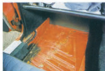
Front footwells corrode badly. This one has been patched, which is fine if done well.
