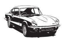
In November 1970 the GT6 Mk3 was launched. In line with the Spitfire MkIV, the tail was "chopped-off" and the bonnet flattened out. The rear roof line of the GT6 was altered and the petrol cap and door handles ceased to protrude. The US market being the largest customer was all important to Triumph and in 1972 to meet US emission regulations the US specification cars saw a change in carburettor, piston, ignition, distributor and camshaft design reducing the cars power to 95bhp.
