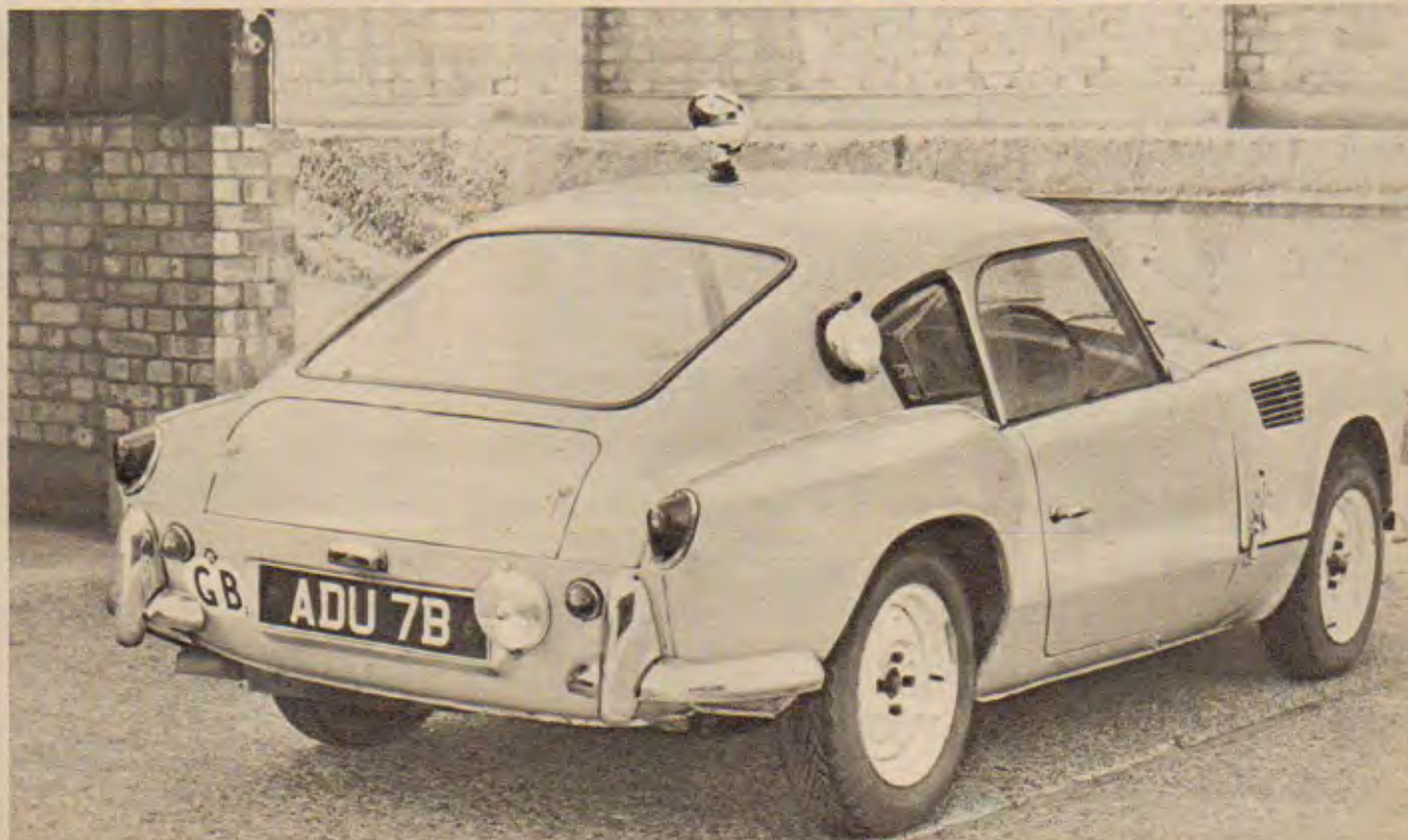
Left: Team-mate ADU 6B runs through northern France in last year's Monte Carlo Rally. We have been testing ADU 7B. Below: The little coupés look very pretty with their fast-back roofline. There is a powerful reversing lamp for "wrong slotting" and a signpost lamp on the roof
