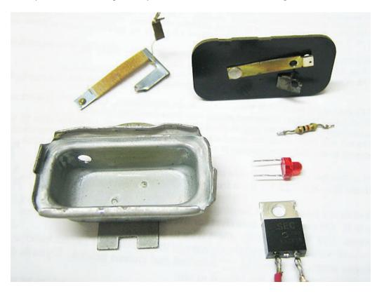
Upper left: the resistance-wire wrapped bimetallic element of an old-fashioned thermal Voltage Stabilizer.
