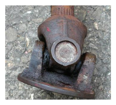
With all of the circlips removed, hold the shaft in one hand with one of the bearing caps in the flange uppermost. Strike the flange downwards with the soft faced hammer, popping the bearing cap upwards. Once there is sufficient of the cap outside the flange, turn the shaft through 180 degrees and repeat for the opposite bearing cap. You will now be able to remove the flange from the UJ and remove the caps by gripping their ends firmly in the vice.
