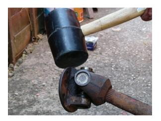
Similarly remove the bearing caps from the yoke by supporting the bare ends of the spider across the vice, while striking down on the yoke inboard of the cap. With a little practice, this method gets a UJ stripped in 5 minutes, though that doesn't include the circlips - no shortcuts with those I'm afraid.
