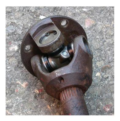
Remember that unlike the propshaft UJs, those on the halfshaft must be set tight. A correctly installed halfshaft UJ will be quite tight but smooth when the flange is moved by hand - this is off the car of course. Triumph specialists will be able to supply circlips in various thicknesses to take up any endfloat across the UJ. The factory supplied circlips in 4 different thicknesses, but most specialists have settled on just 2 sizes, .0615" and .0645".
