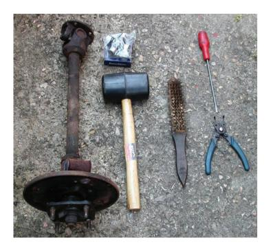
I remove the UJs using a slightly modified version of the technique favoured by John Kipping. The technically correct method of pressing out each bearing cap in a vice may be fine with new components, but it can be a nightmare with anything which has seen 40 years of use.
