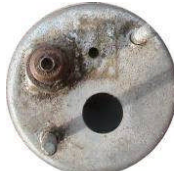
Rear view of Smiths Bourdon tube pressure gauge
