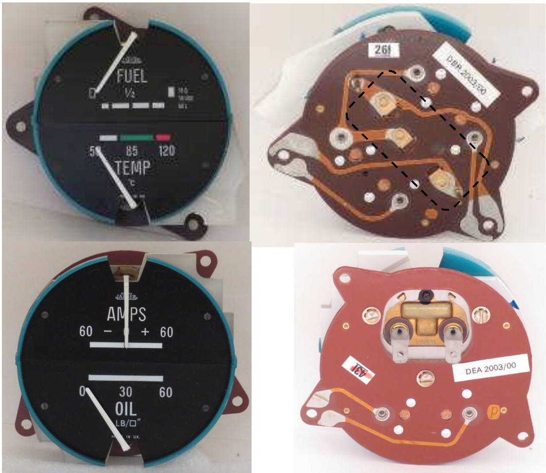
FIGURE 13: Front and rear views of the DBR 2003/00 (top) and DEA.2003/00 (bottom) dual electric gauges fitted to some Rover cars.
