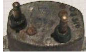
FIGURE 25: Bullet style terminals on TE gauge.
