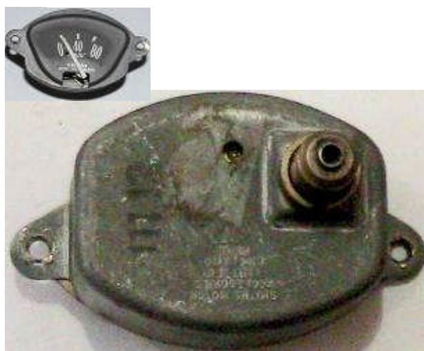
FIGURE 5: Quadrant style oil pressure gauge.
