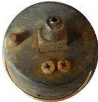
Rear view of Smiths diaphragm pressure gauge
