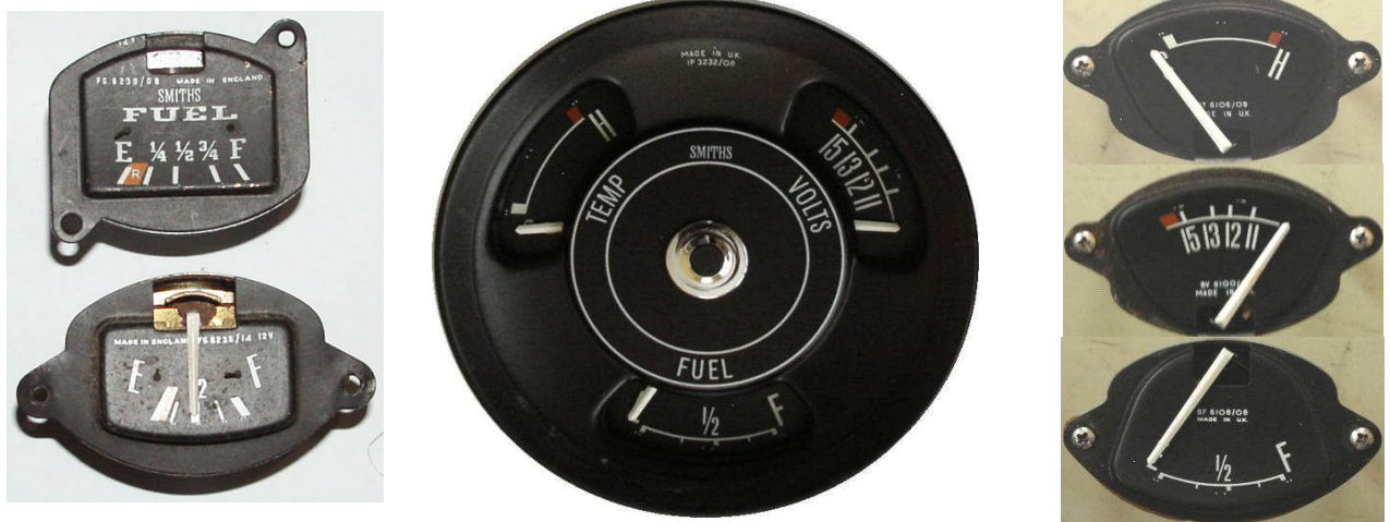
FIGURE 2: Photos showing the two styles of "quadrant" gauge on the left and to the right an instrument panel from a Triumph 2000 Mk II. The parts listing for this Triumph instrument panel are:
