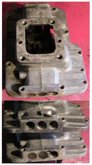
Top photo shows rear of early cover. The bottom photo shows the rear views of a late (upper) and early cover (lower).
