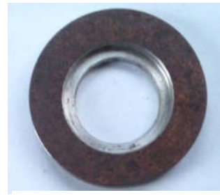
Finished housing support plate.
