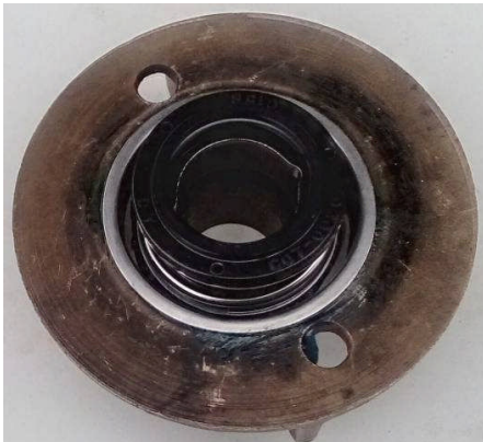
Seal fitted to an impellor ready for assembly.
